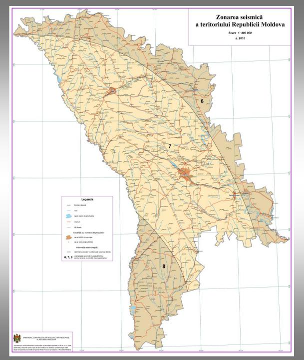
The seismic zoning map of Moldova Republic was adopted by the *Ministry of Regional Development and Construction* in 2010, and approved for practical use (seismic design and construction).
