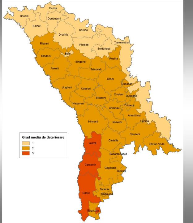
Seismic risk map of Moldova Republic has been created in 2013. It was elaborated for scenario earthquake (like 10.11.1940) in terms of the average degree of damage for each district.
