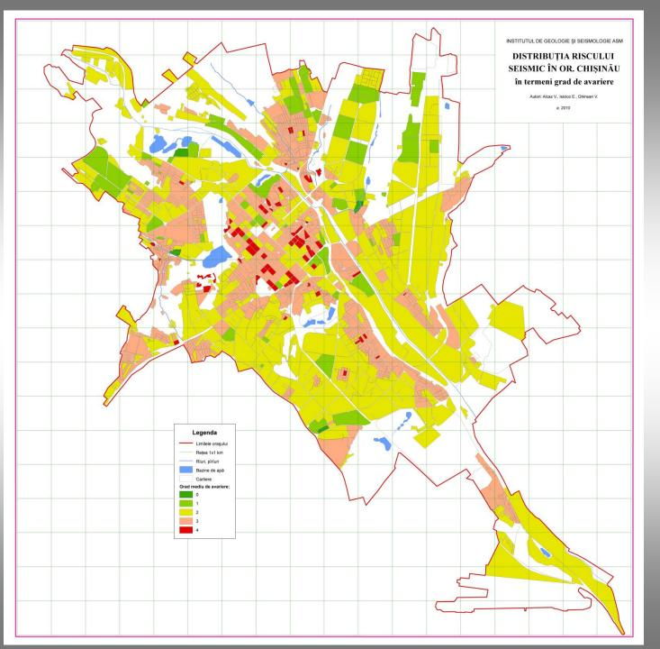
Seismic risk map of Kishinev city has been created in 2009. It was elaborated for scenario earthquake (like 10.11.1940) in terms of the average degree of damage for each quarter of the city.
