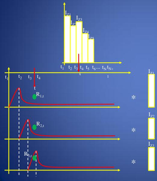
As a result of dealing with the governing second-order linear partial differential equation, it is required to carry out a solution for each hourly rainfall data in rainfall sequence, thus leading to the superposition of pore pressures generated due to each rainfall data.
