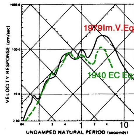
Notice the **different response** of the structure due to different accelerograms with the same (0.36g) PGA.
